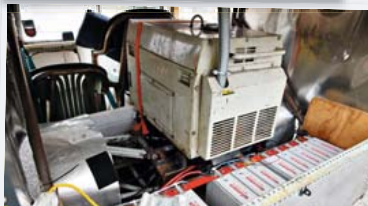
Power comes from a cluster of 13 12V batteries at the rear of the car
