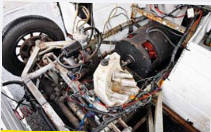
Milk-float motor is more securely fixed than the range-extender generator
